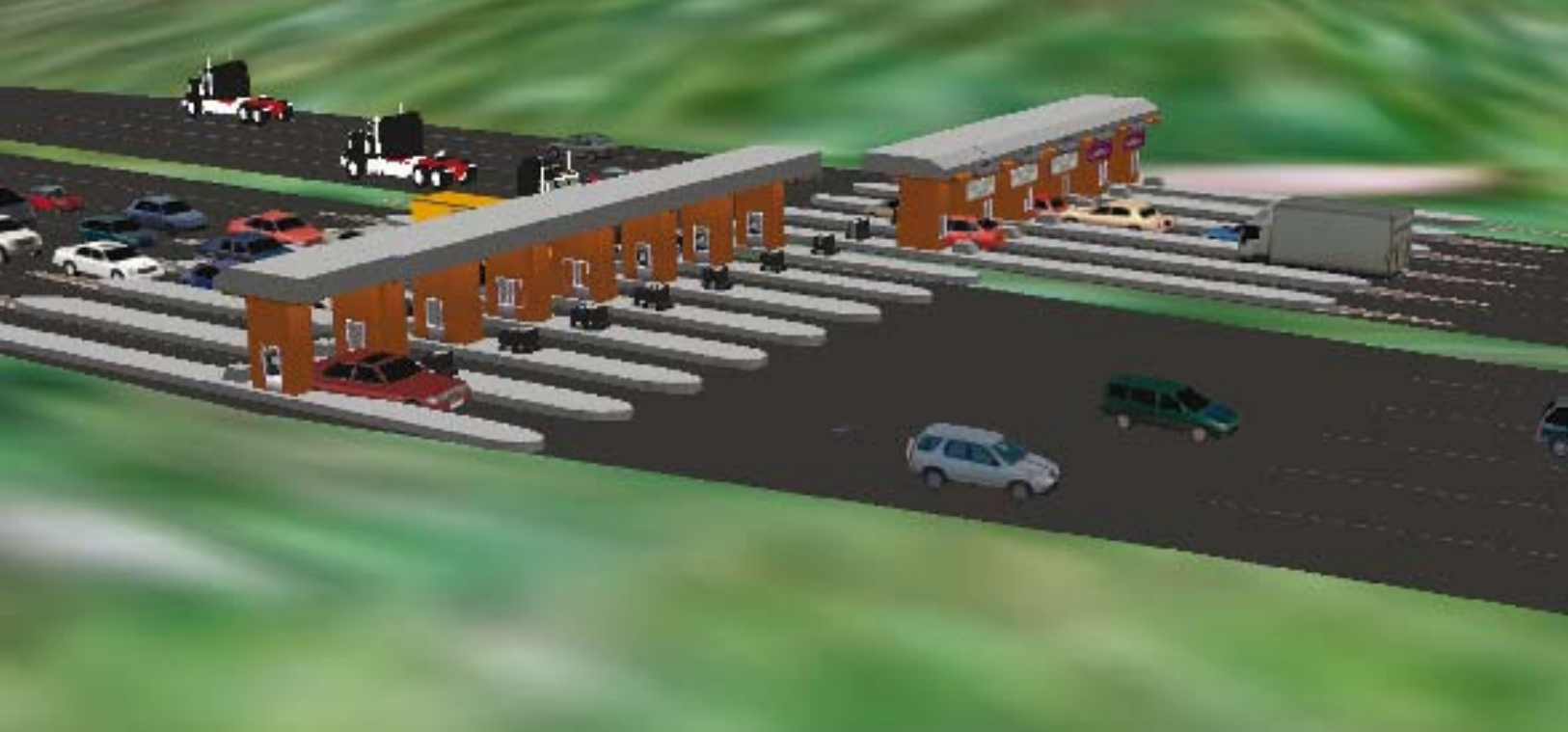
⌚ This image portrays a 3D toll plaza with multiple toll booths. When modeling plazas with multiple booths, looking at approach lane definition is crucial
