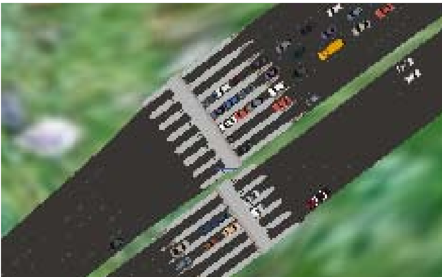
⬆ Microsimulation is a useful tool for the tolling industry. This image shows a 2D view of a toll plaza, demonstrating the delay that is caused to those drivers who are using traditional payment methods
