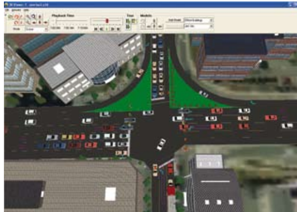
SimTraffic simulates signalized intersections, unsignalized intersections (including roundabouts) and the interaction that occurs
